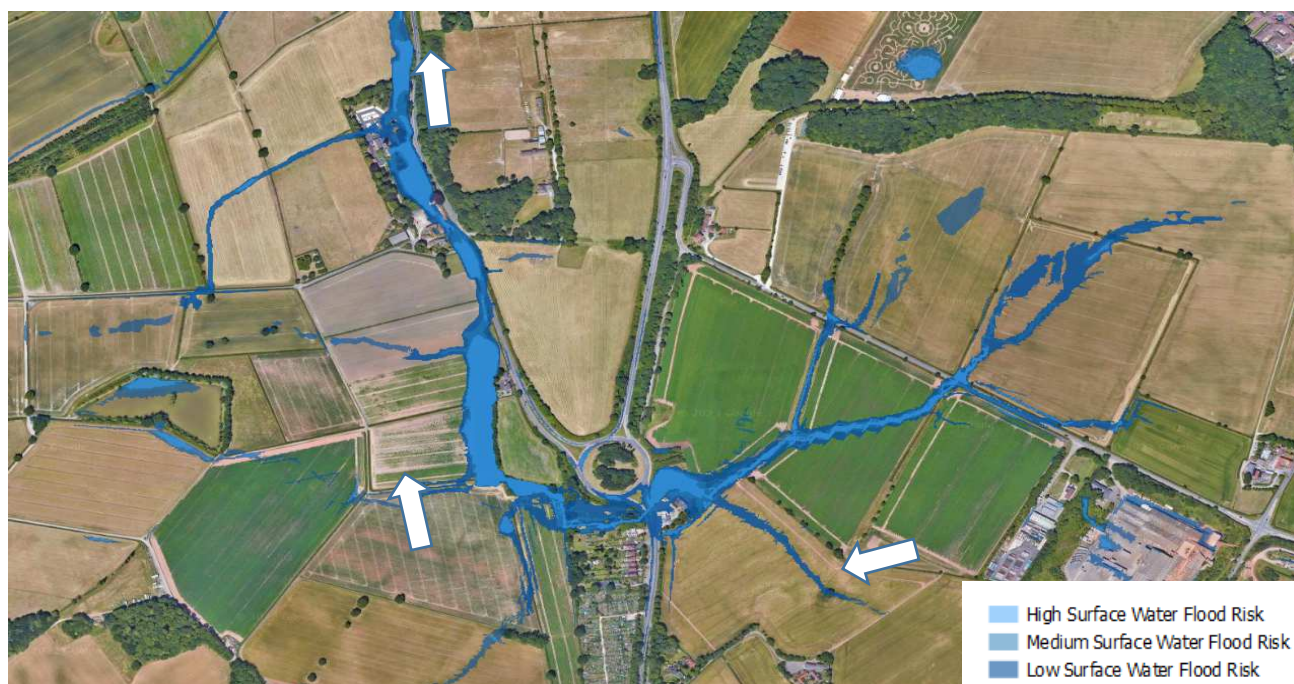
Figure 4. Surface water flood mapping for Mansfield Road. Data supplied by Environment Agency.
