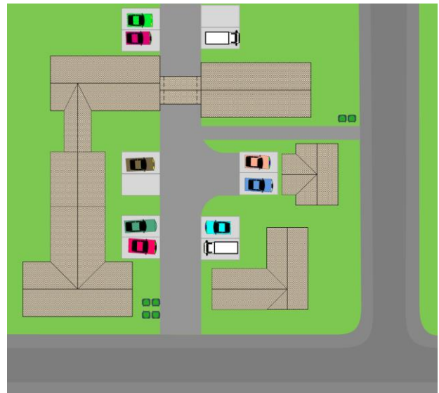
Figure 1.2 Easily accessible car parking with good natural surveillance and association with dwellings
