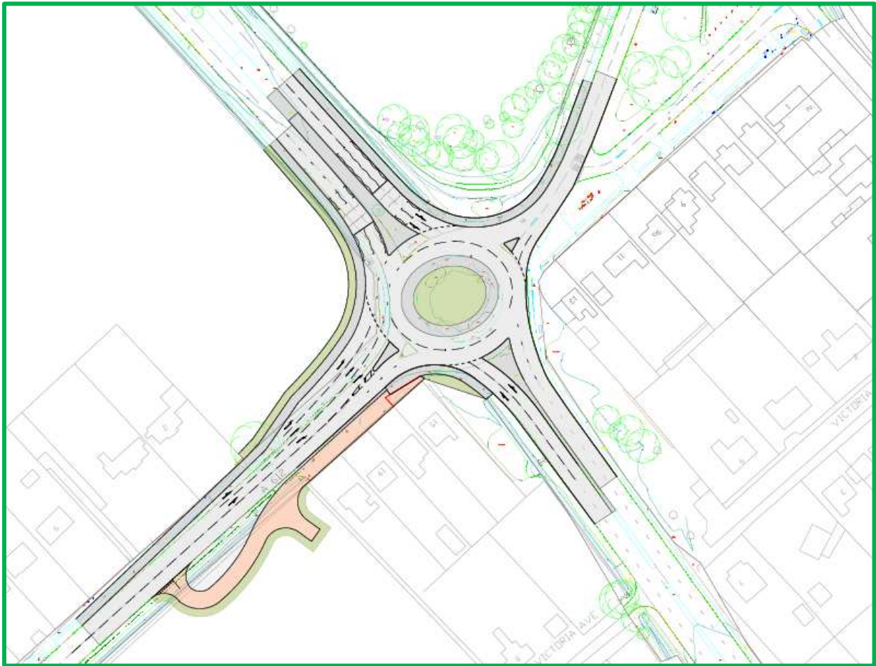
Figure 5-4 Lowdham roundabout scheme
