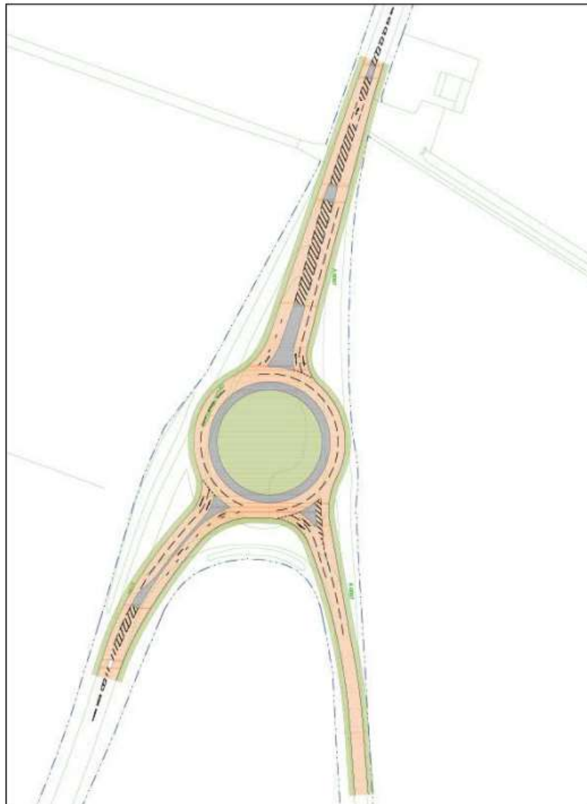
Figure 12: Conventional Roundabout option for Warren Hill junction
