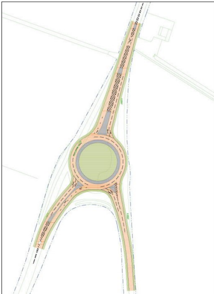
Figure 12: Conventional Roundabout option for Warren Hill junction
