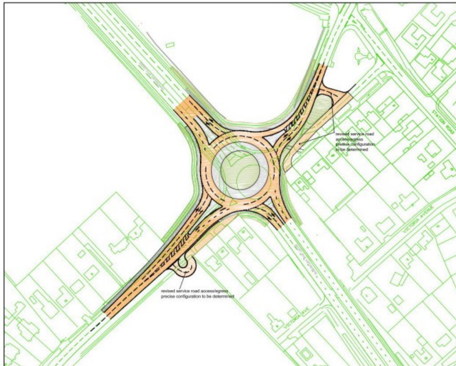
Figure 14: Enlarged conventional roundabout option at Lowdham Roundabout
