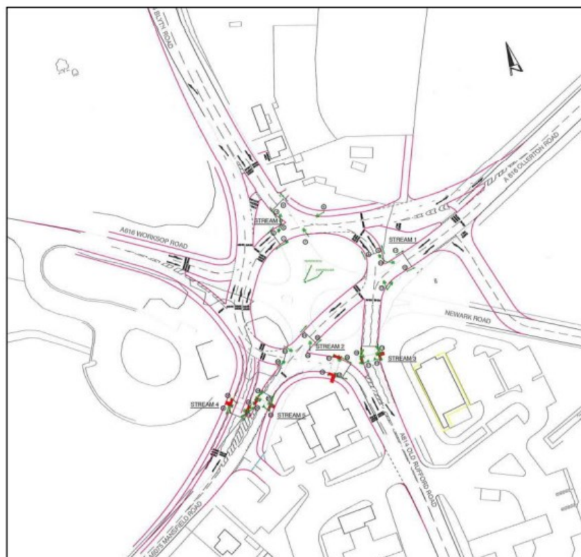
Figure 7: Traffic Signals option for Ollerton Roundabout
