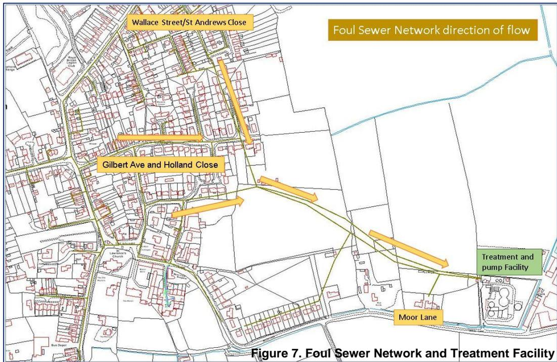
Figure 7. Foul Sewer Network and Treatment Facility
