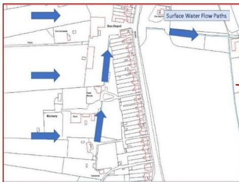
Figure 5. Flow paths for Leake Road area
