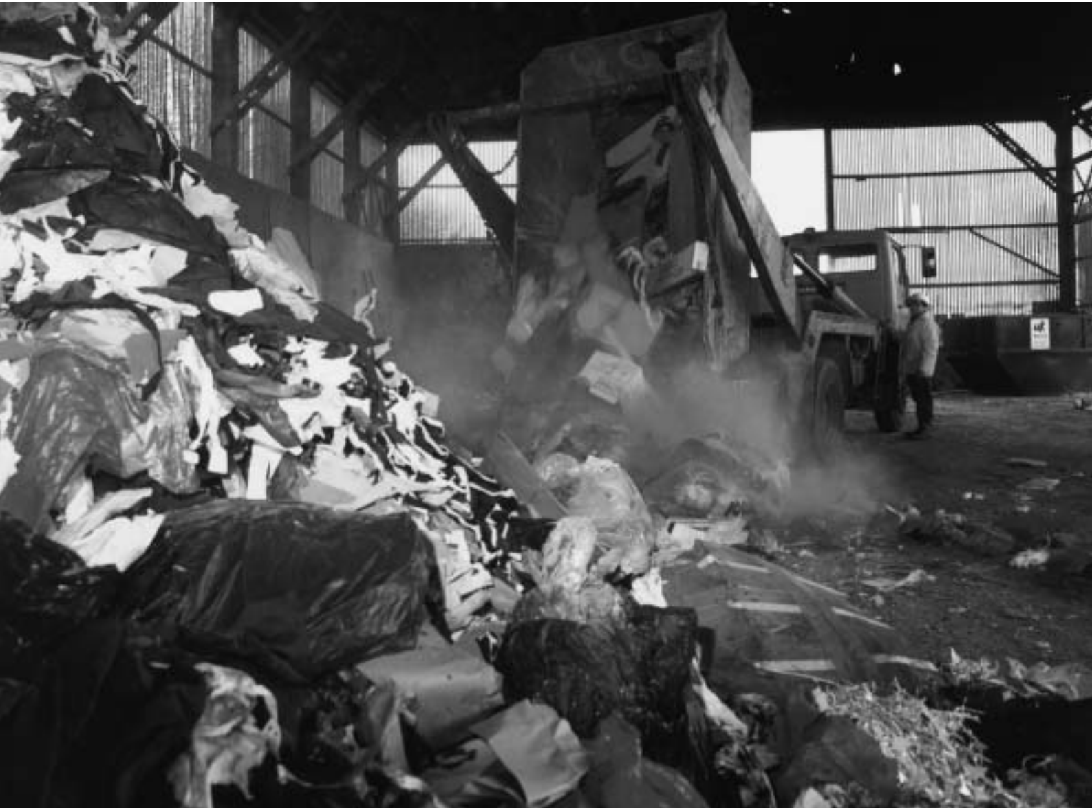
A typical general waste transfer section. Waste is collected from a wide range of sources before being sorted and bulked up for disposal or recycling.
