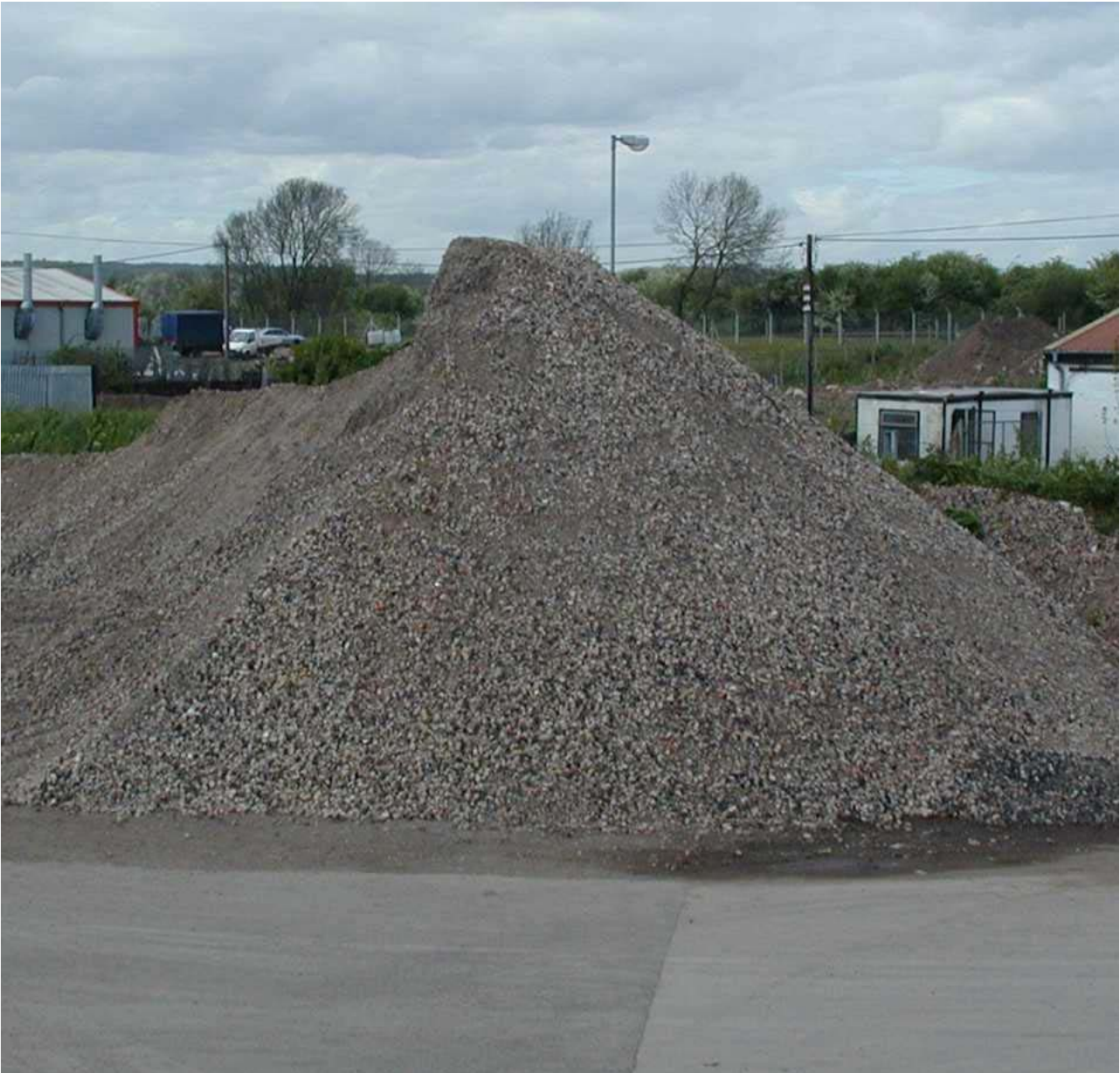
Pile of crushed bricks at Tarmac's recycling facility at Colwick Industrial Estate
