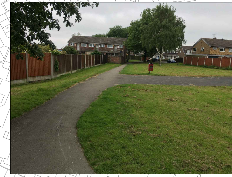
Existing footway to be widened to min. 3m for shared use cycle footway
