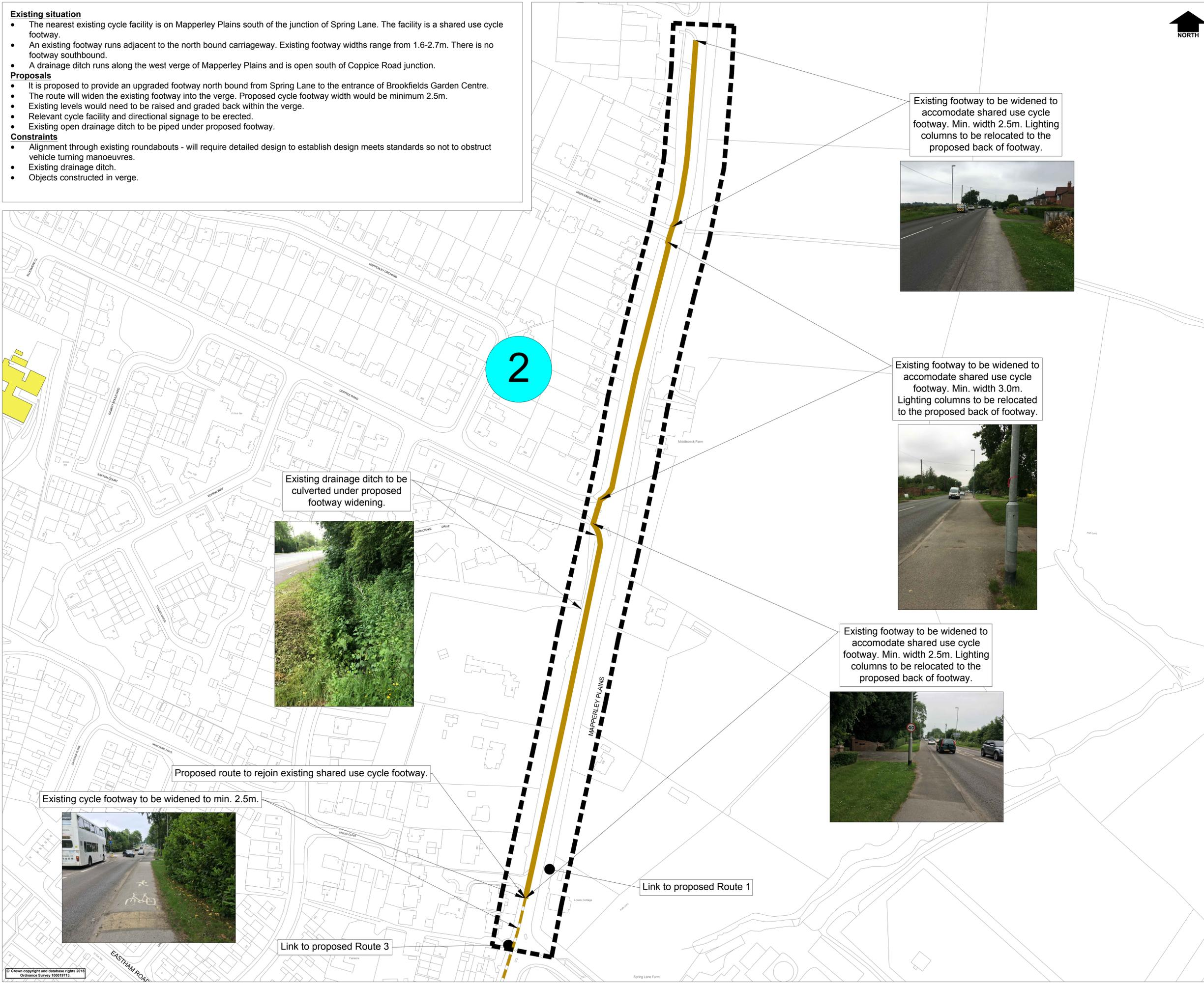
Existing footway to be widened to accommodate shared use cycle footway. Min. width 2.5m. Lighting columns to be relocated to the proposed back of footway.
