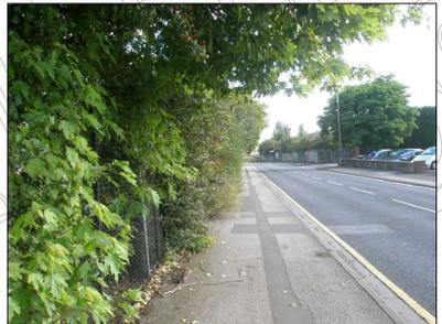
Footway to be widened to accommodate proposed bus shelters and real time poles
