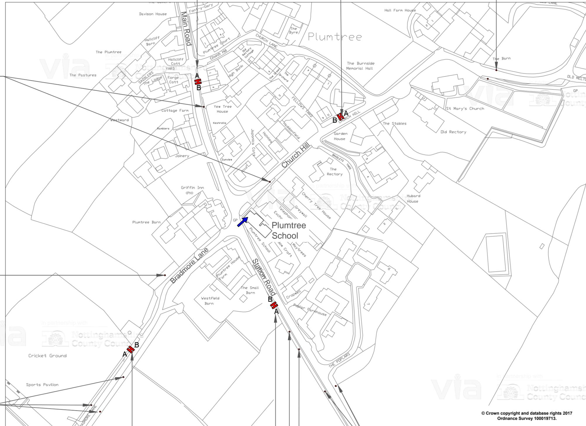
Proposed signs mounted back to back on 1 no 76mm post, 2.3m mounting height. Post to be installed to rear of footway.
