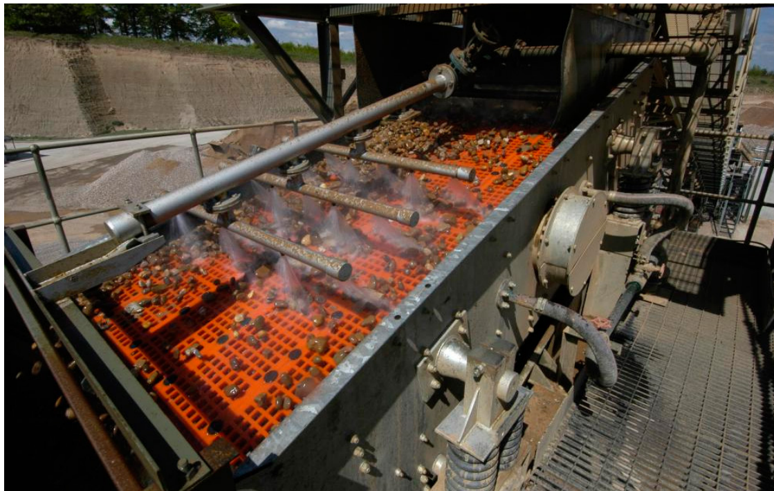
Washing and screening sand and gravel.
