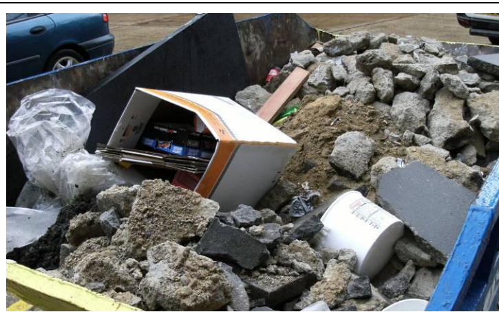
Figure 4.1: Typical incoming mixed skip waste from a small construction site, where the skip was accessible to the public. The recovery of otherwise clean soil and 'hard' CDEW will be complicated by the inclusion of both other CDEW and non-CDEW.
