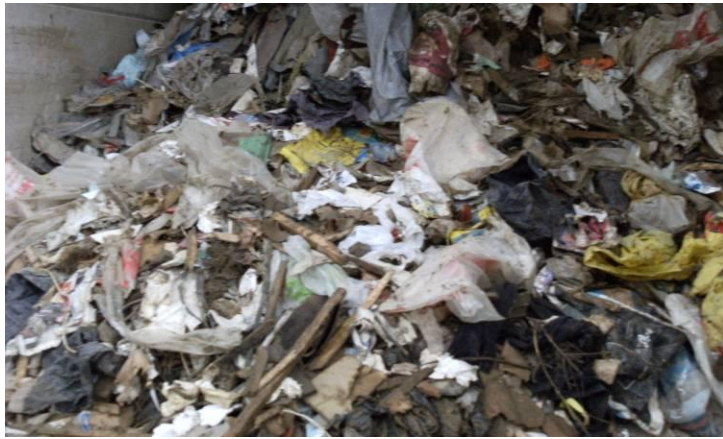
Figure A8.Site14.6: Residual waste from the picking station. Much of this is very dirty timber, card and soft plastics.
