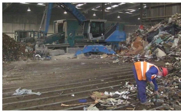
Figure A8.Site8.2: Hand picking of cable, wood and plasterboard. Grab removing large items before screening.
