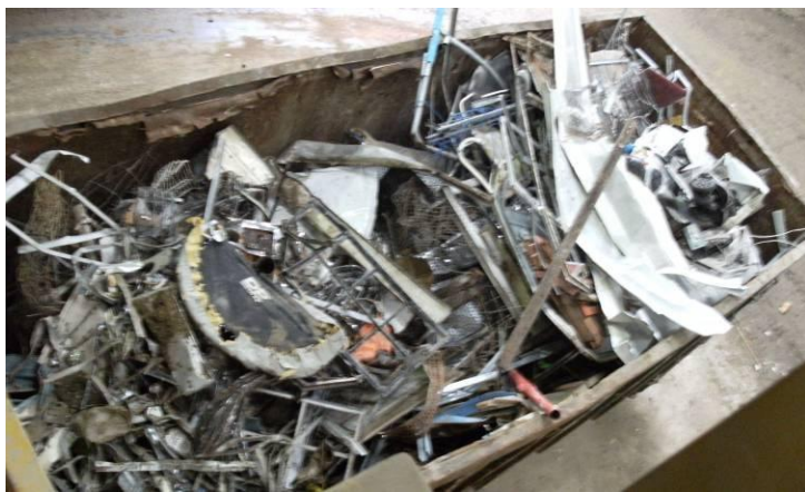
Figure A8.Site14.7: Metals removed by the magnet (after the picking station).
