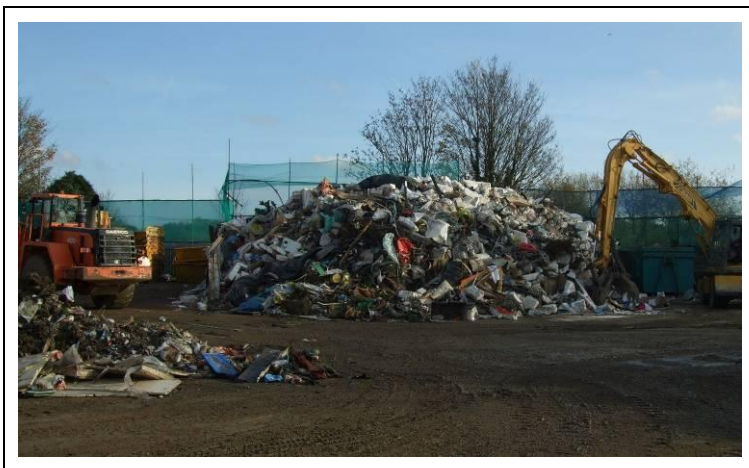
Figure A9.Site13.1: To the left is a pile of incoming waste being hand picked. The main pile is residual waste which is dispatched to another waste treatment facility for further processing.
