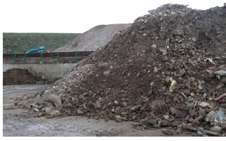
Figure 4.2: Incoming waste dominated by soil, from a construction site where the operator had kept to a minimum the inclusion of 'contraries'.
