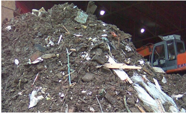
Figure A9.Site28.1: Incoming CDEW – mostly soil, but with significant levels of contaminants mixed in.
