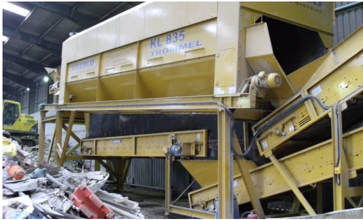
Figure A8.Site14.2: Trommel screen and conveyors. One conveyor carries the fines outside; the other takes the residual waste to the picking station.
