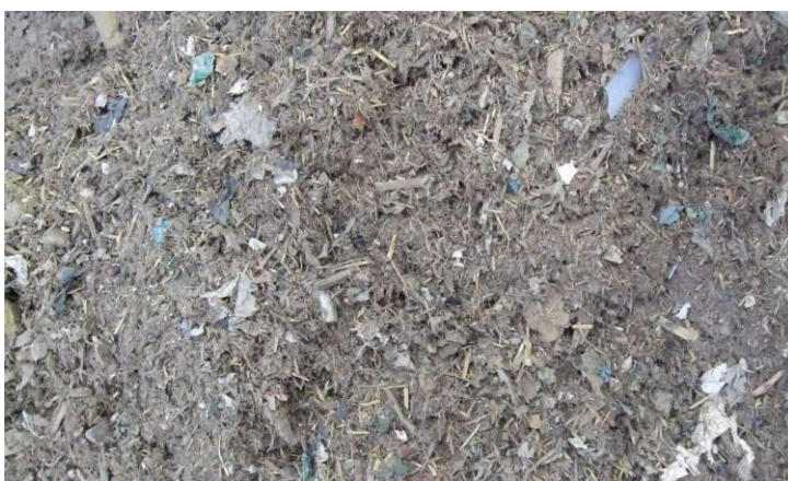
Figure A8.Site8.5: Intermediate stage waste. More soil will be screened out before the residue becomes RDF.
