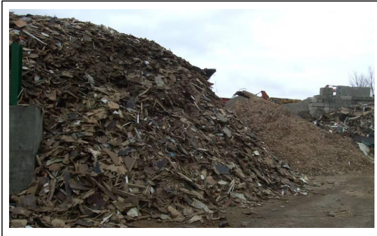
Figure A8.Site19.6: Separated wood board ready for chipping. This will be burned as RDF.
