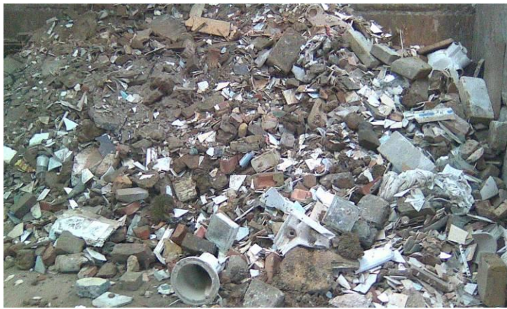
Figure 4.4: Mainly 'hard' incoming CDEW (from the demolition process), but with some soil, wood and plastics mixed in.
