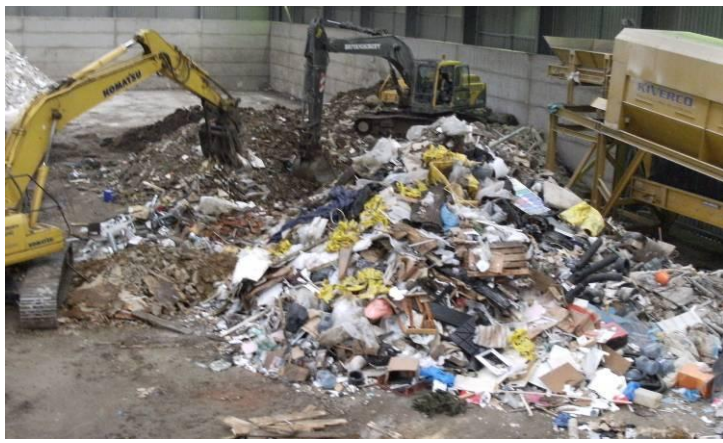
Figure A8.Site14.1: Heavily mixed incoming wastes being sorted by grab, with the residual fraction being loaded into the trommel screen's feed hopper.
