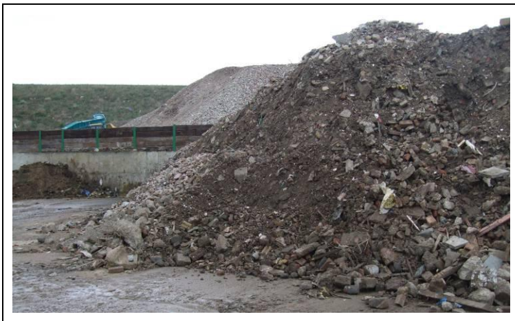
Figure A8.Site19.1: Incoming waste with a high inert content, waiting to be screened.
