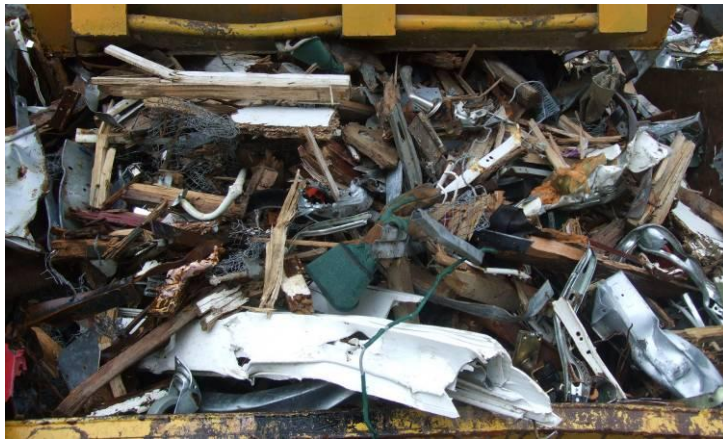
Figure A9.Site27.5: Mixed contaminants screened out of soil and hardcore.
