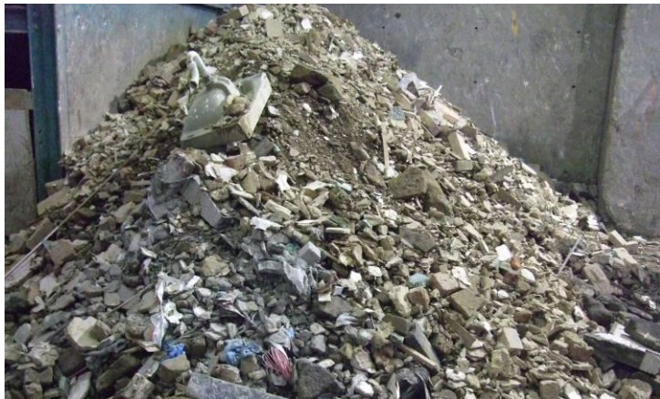
Figure A9.Site24.1: Incoming CDEW after hand picking. This waste will be screened next.
