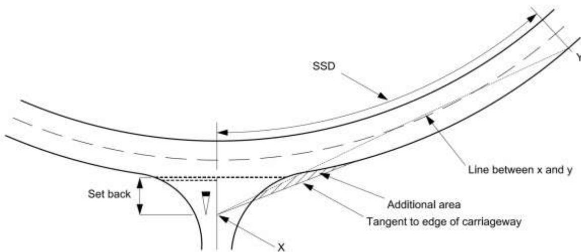
Where the line between points X and Y falls partially within the major road carriageway, an additional area shall be added to the visibility splay formed by drawing a line from X to a point tangential to the nearer edge of the major road running carriageway.
