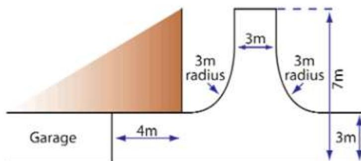
The area required for turning should not form part of the overall space required for parking. Driveway width subject to change, see Driveway widths above. Larger turning areas may be required if it is necessary to accommodate delivery vehicles.
