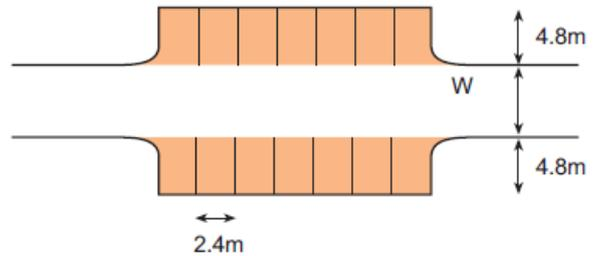
The width ( $W$  above) needed to access echelon or perpendicular spaces conveniently, depends on the width of the bay and the angle of approach. For a 2.4m wide bay, these values are typically:
