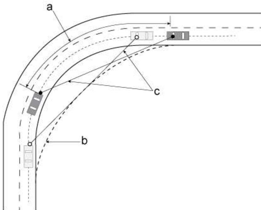
3.3.5 Forward visibility is the distance a driver needs to see ahead to stop safely to avoid an obstruction in the road. The minimum forward visibility required is equal to the minimum SSD. It is checked by measuring between points on a curve along the centreline of the inner traffic lane where 'a' is the forward visibility measured along the centre of the inner lane, 'b' is the visibility splay envelope, and 'c' is the visibility splays.
