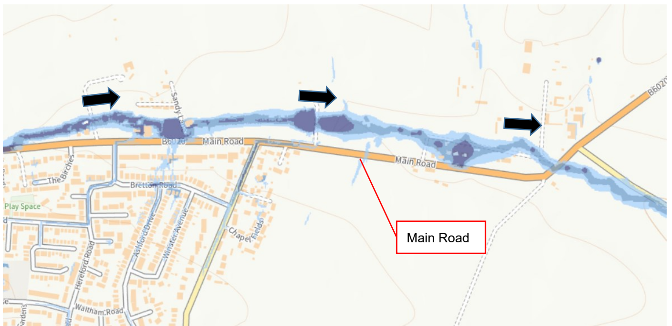
Figure 3. Predicted Surface Water Flood Extents – Main Road
