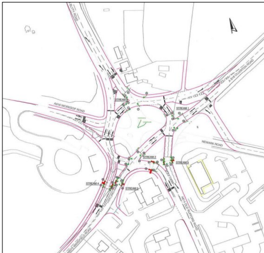
Figure 3: Traffic Signals option for Ollerton Roundabout
