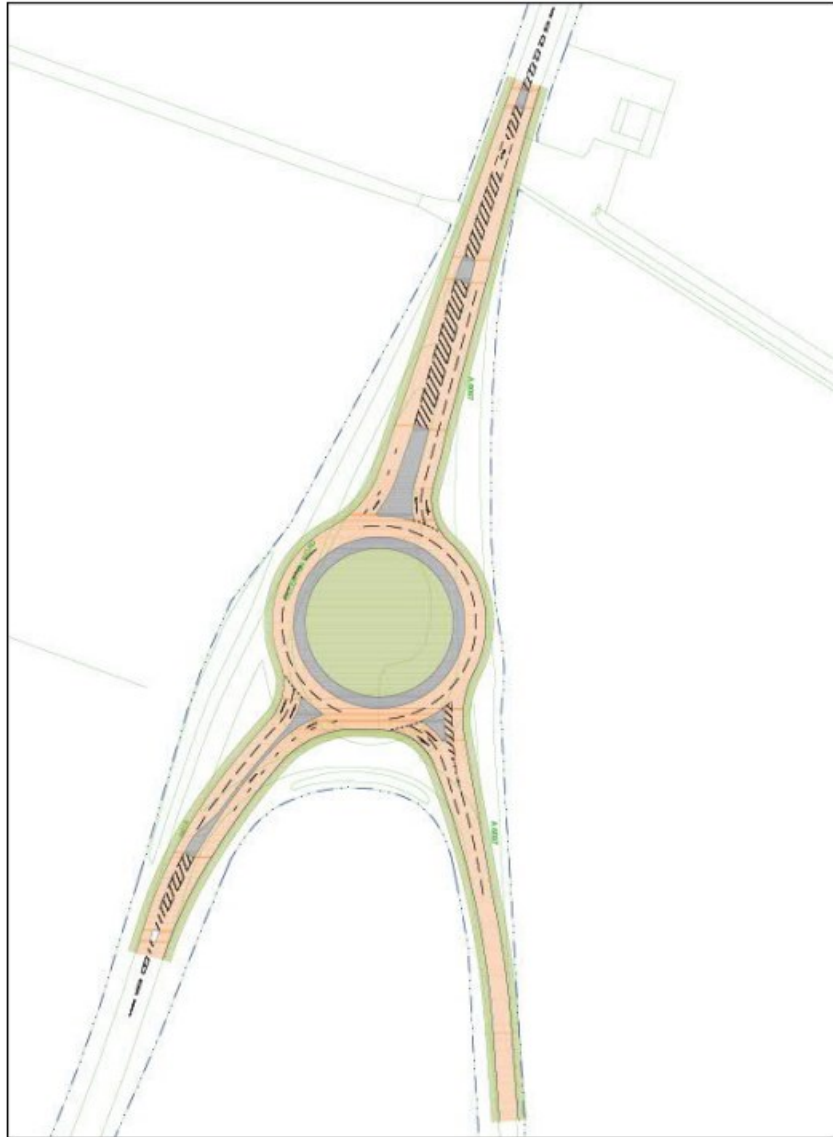
Figure 6: Conventional Roundabout option for Warren Hill junction
