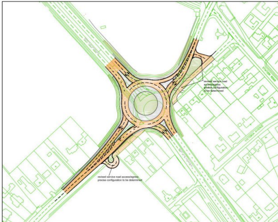
Figure 8: Enlarged conventional roundabout option at Lowdham Roundabout
