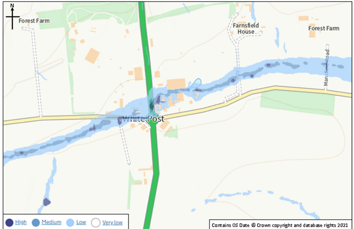
Figure 5-2: White Post Roundabout Extent of Flooding from Surface Water
