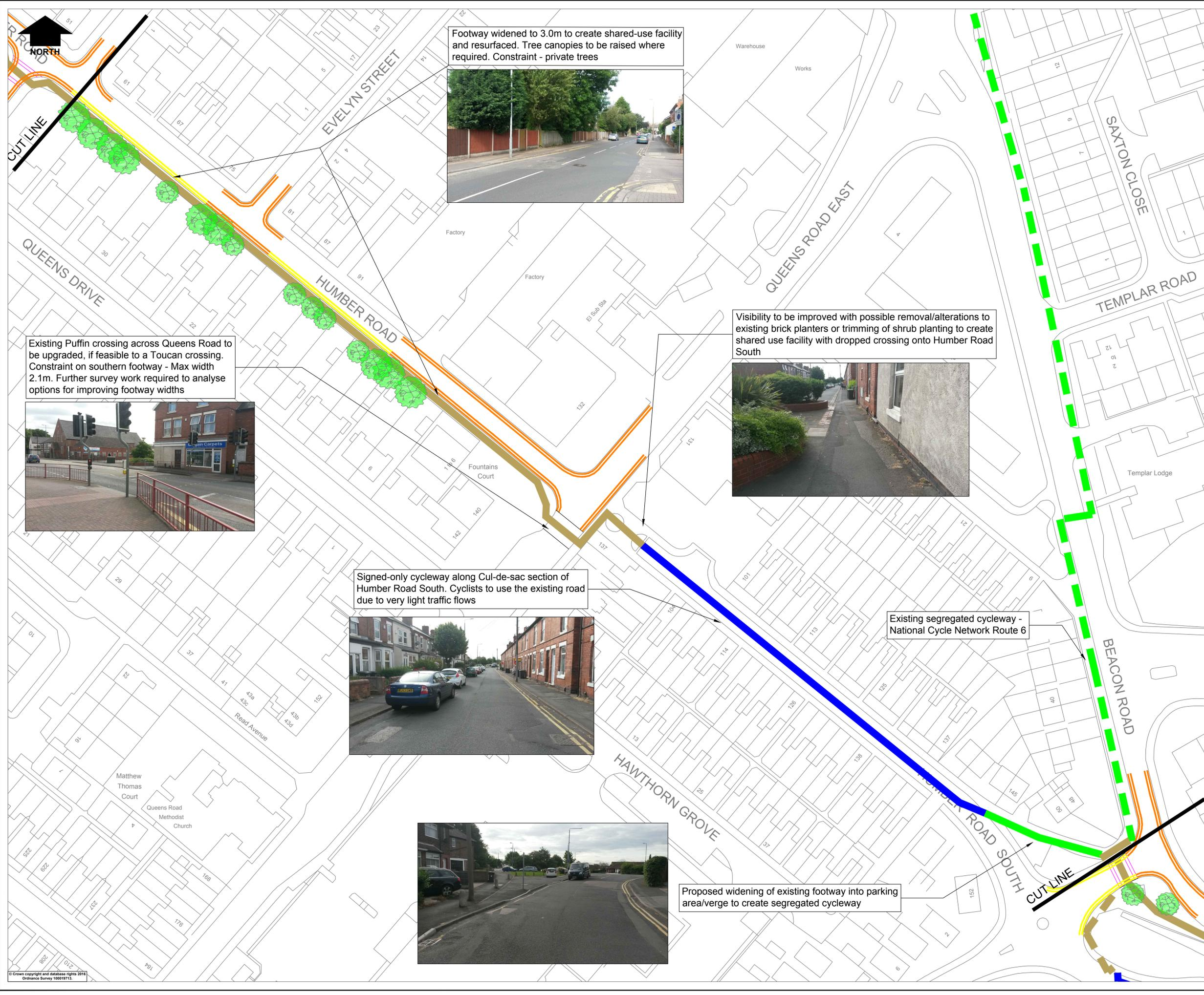
Footway widened to 3.0m to create shared-use facility and resurfaced. Tree canopies to be raised where required. Constraint - private trees
