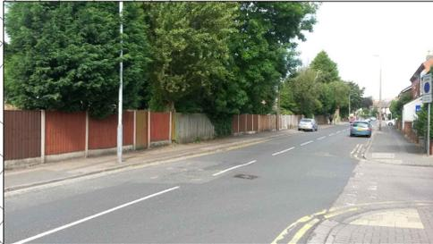
Existing Puffin crossing across Queens Road to be upgraded, if feasible to a Toucan crossing. Constraint on southern footway - Max width 2.1m. Further survey work required to analyse options for improving footway widths
