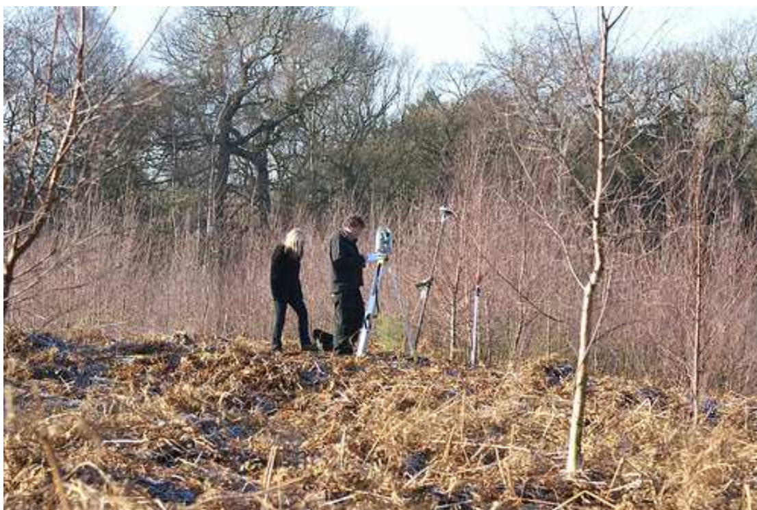
Photograph 7: Community Archaeologists undertaking EDM Total Station survey. Reproduced with permission from Lynda Mallett ©.
