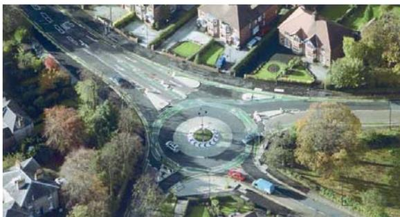
**Photo 7.4** Cycle lanes at a roundabout.
