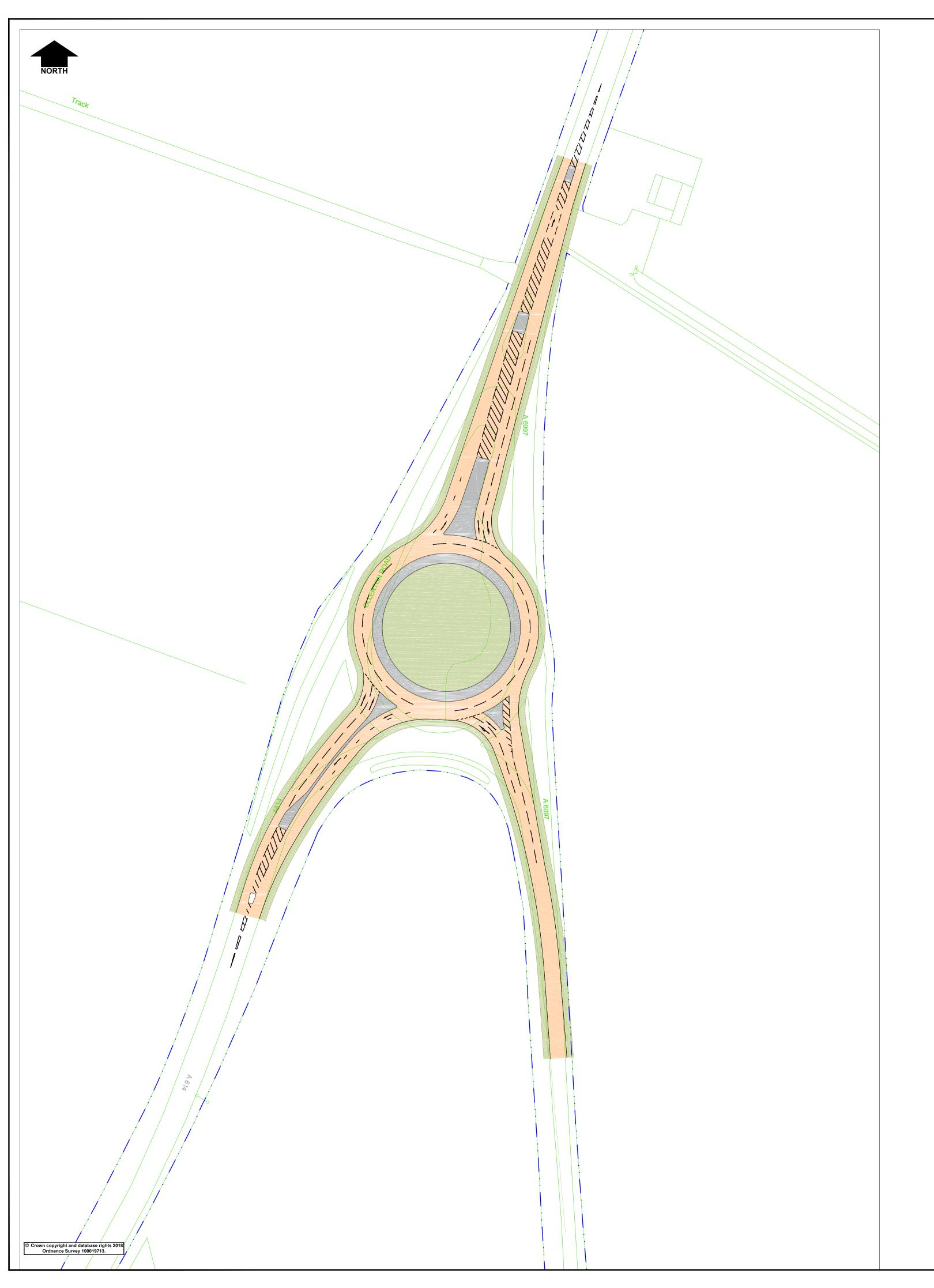
1. This drawing shows the replacement of the existing junction form with a new 85m ICD roundabout.
