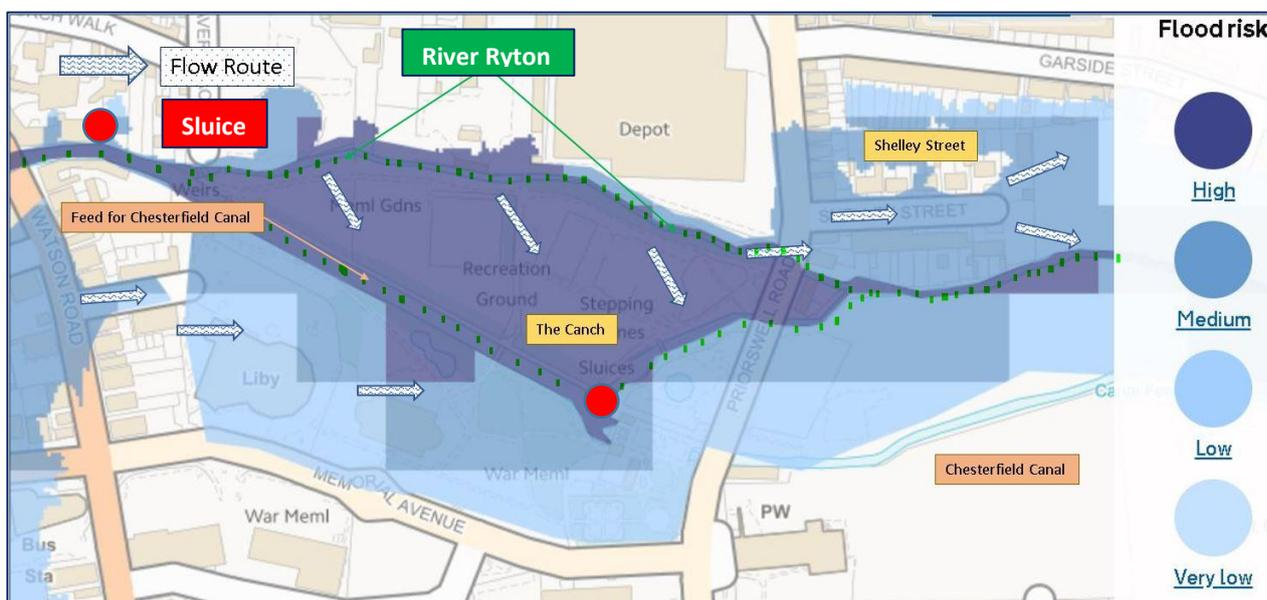
**Figure 6. Flood Extents and Flow Routes in The Canch area**
