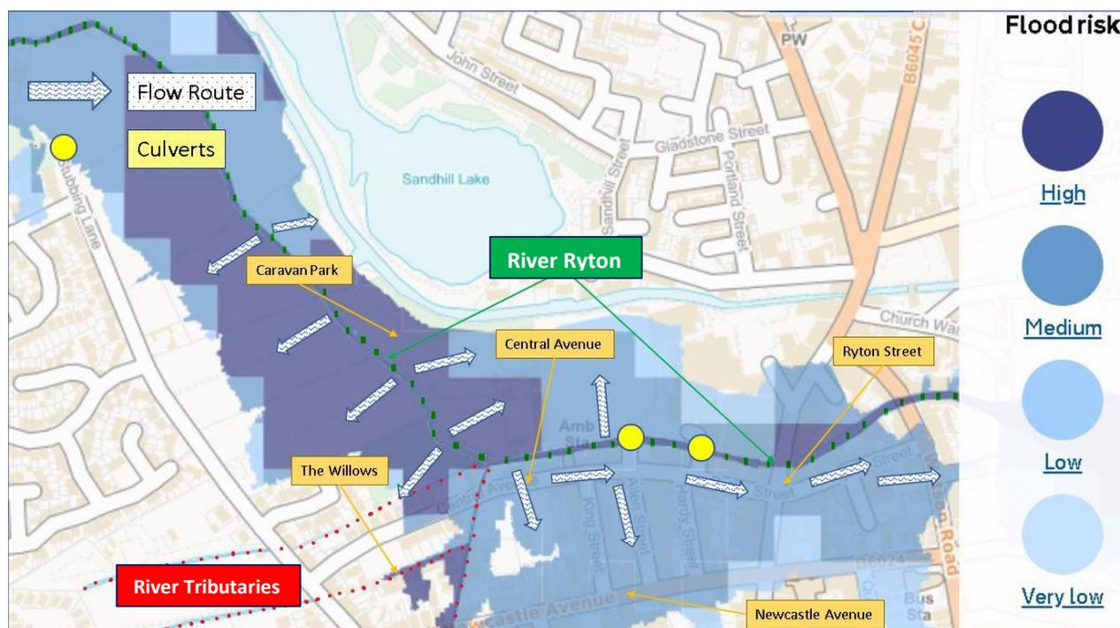
**Figure 5. Caravan Park and Culvert Location showing flow paths from overtopped River.**
