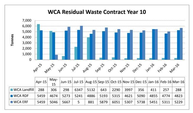
All residual waste from the districts of Ashfield and Mansfield was transferred to Alfreton transfer station where the waste is processed into a refuse derived fuel (RDF).
