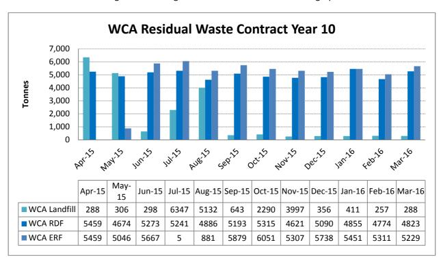
All residual waste from the districts of Ashfield and Mansfield was transferred to Alfreton transfer station where the waste is processed into a refuse derived fuel (RDF).
